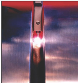
Cutting Edge Narrow-Groove Pipe Welding Technology
