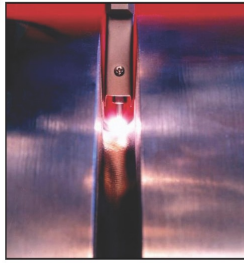
Cutting Edge Narrow-Groove Pipe Welding Technology
