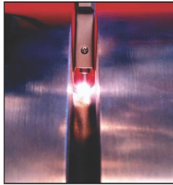
Cutting Edge Narrow-Groove Pipe Welding Technology
