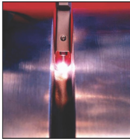
Cutting Edge Narrow-Groove Pipe Welding Technology
