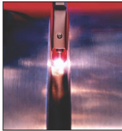
Cutting Edge Narrow-Groove Pipe Welding Technology
