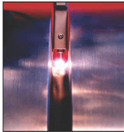
Cutting Edge Narrow-Groove Pipe Welding Technology
