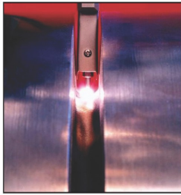
Cutting Edge Narrow-Groove Pipe Welding Technology
