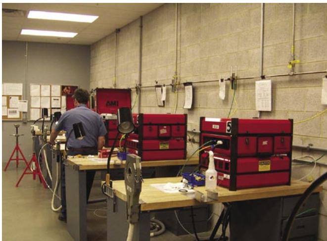
**Photo 2:** Five of the six Arc Machines orbital welding power supplies equipped with water cooling units in the welding room; note documents at each weld station that travel with the weld assemblies.
