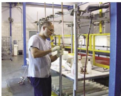
**Photo 7:** A technician in the SBBIS electropolishing facility prepares a part for electropolishing. This “hands-on” process is still operator dependent.
