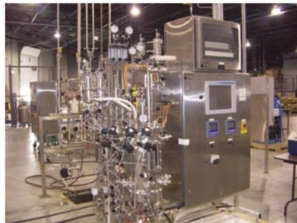
**Photo 1:** Fermentor with associated control system nearing completion on the manufacturing floor
