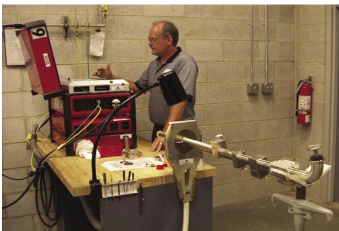
**Photo 3:** A welding operator initiates an orbital weld. A pipe stand is used to support the tubing assembly. The built-in purge system shown above the power supply delivers high-purity argon gas for purging the weld in the enclosed type weld head and to the tubing ID.
