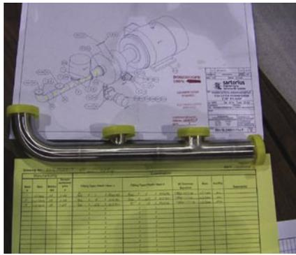
**Photo 6:** A welded assembly with its control document (yellow) and weld map showing location of the assembly with each weld numbered on the CIP pump for a 750-L fermentor
